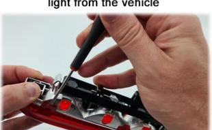
Carefully lever these up to release the light strip from the red lens
