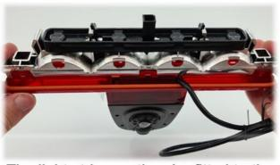
The light strip can then be fitted to the camera, then screwed on to vehicle
